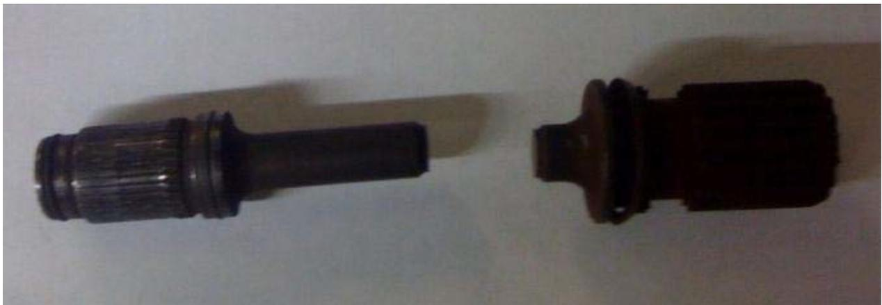
Bombardier BD100-1A10, Sheared Generator Spline Shaft, ATA 2421
